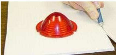
Once you've chosen a lens to reproduce, choose a material to make your mold base and box out of. Here you see us using some inexpensive corrugated plastic. It is easy to cut with an Excel knife and can be used for the base as well as the sides if you so choose.
