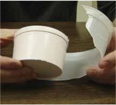
Allow the rubber to cure overnight and then remove the mold from the mold box.
