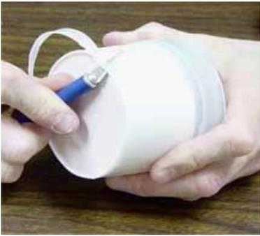
Using the rubber as a guide, trim the bottom of the mold box so it sits nice and flat.
