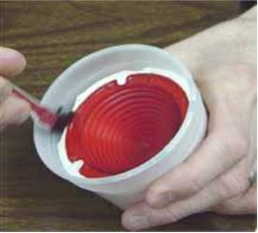
If you are using Alumilite's Rubber to Rubber Mold Release, we recommend waiting 5-10 minutes between coats and putting at least 2 if not 3 individual coats on to make sure the rubber does not stick. Also, make sure to shake the bottle well before using.
