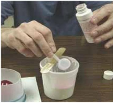
Once you've added the catalyst you are now ready to mix. The work time of the High Strength 2 is approx 45 minutes and the demold time is 12-18 hours.
