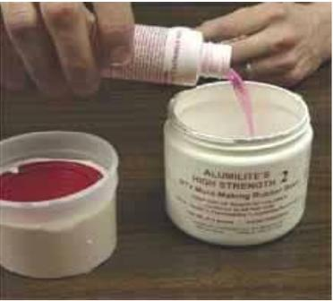
After calculating the volume required for the second half of the mold the same way we did for the first we realize we need approximately the same amount of rubber for the second half of the mold. Since we already used a 1/2 lb out of the 1 lb kit, we can simply dump the remaining catalyst in the base container of the 1 lb High Strength 2 kit.
