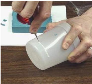
We chose to use a plastic container that leaves 1/4" clearance between the container and the lens as our mold box. In this picture you can see that we cut the bottom of the container off so we can pour through that hole. Keep your mold box (whatever you choose to use to construct it) tight to your piece to decrease the amount of rubber needed to make the mold.
