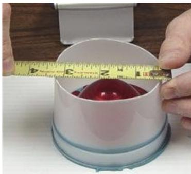
Next you will need to calculate how much rubber you need to fill the mold box minus the volume the lens. To calculate the volume of a round mold box you need to know the radius (which is half the diameter or the length across the box). Visit the [Material Calculator](#) page on this site to calculate the amount of silicone and resin you will need for your part.
