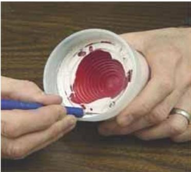
Once you have removed every single spec of clay, trim off the rubber that may have flowed underneath the lens with a sharp knife.
