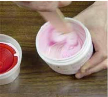
Mix the rubber thoroughly. Be sure to scrape the sides and bottom extremely well. This is very important when mixing in a container with a lip. The lip will limit your access to the side walls so make sure to scrape them vertically as well as horizontally.
