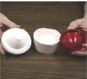
Remove the original lens and you are now ready to start pouring parts in your high tear strength silicone rubber mold that will produce exact replicas of your original.
