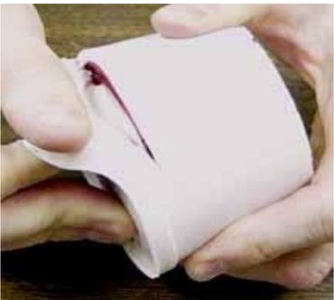
Once you've removed the mold box, find the parting line (area where the two halves of the mold meet) and begin separating the two halves. Do not use a knife. The mold halves should separate using just your fingers.
