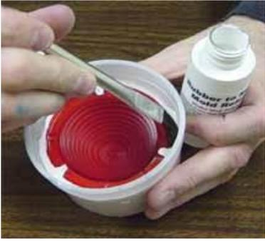
Once you have cut locators in the first half of the rubber mold, use Alumilite's Rubber to Rubber mold release or Alumilite's UMR to make sure the second layer of rubber will not bond to the first. The mold release only needs to be applied to the rubber and not to the part to prevent witness marks on the lens itself.
