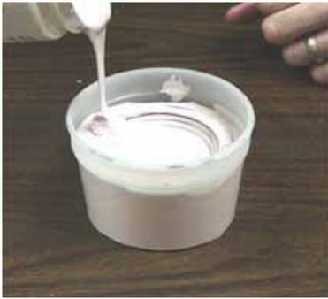
Once you've painted in a skin coat, simply pour the remaining rubber into the mold.
