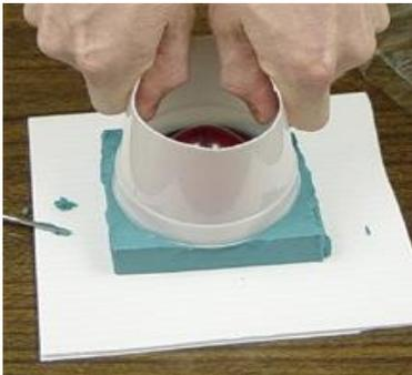
Once we have cut the container's bottom off, we flip the container over and press it into the clay around the lens leaving a 1/4" gap between the lens and the mold box.
