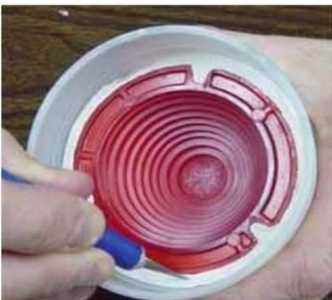
Using an Excel knife, cut some locators on the outside of the silicone rubber to the mold box. Put your knife at an angle and cut a wedge shape locator approximately an inch long. Do not allow the knife to get to the original part. You can see one that is already cut at approximately the 11:00 position. It is slightly more shady and will allow the second half of the rubber mold to flow in that channel and locate the two halves.
