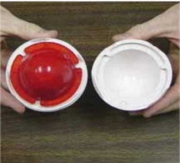
This picture shows you the two halves of the rubber mold with the lens still inside. If you look closely on the outside of the mold edge, you can see the locators that will line up your mold halves in the correct position.
