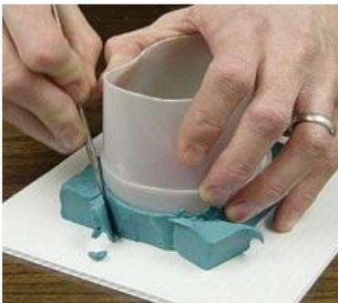
Push the container down into the clay as far as you can. Then trim the excess clay around the mold container and continue to press the container down to the piece of corrugated plastic (mold base).
