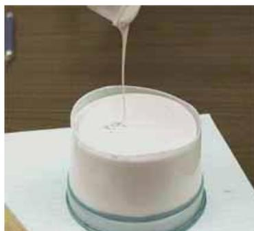
Slowly pour the rubber over the smooth tail light lens. One optional step that is highly recommended on the inside of the mold that you may want to do before pouring the outside is to paint on the initial layer of silicone to make sure your lens surface is perfectly covered with no air entrapment before pouring all the rubber in the mold box.
