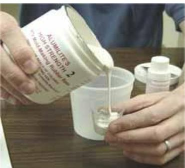
We've decided to use Alumilite High Strength 2 silicone mold making rubber because of its phenomenal physical properties (extremely high tear strength) as well as its low viscosity which doesn't require vacuum to achieve a perfectly good bubble free mold.
