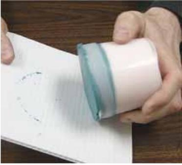
Allow the rubber to cure overnight at room temperature before beginning to work on the second half of your lens mold.
