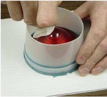
Before pouring the rubber, make sure to clean any fingerprints, smudges, or clay off of the lens.
