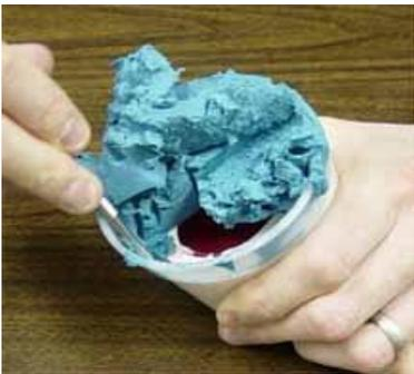
Begin removing all of the clay **WITHOUT** removing the lens or the mold from the mold box. Simply remove the clay and nothing else.
