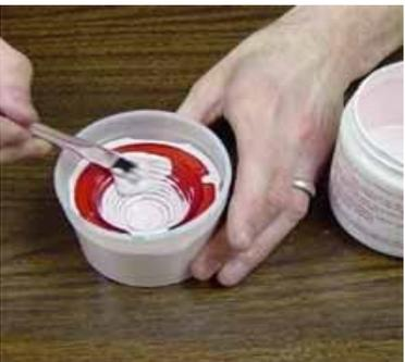
Once the rubber has been mixed well, use a disposable paint or acetone brush to paint on a thin layer of rubber onto the original lens to make sure the rubber is forced into the detailed cracks and crevices of the inside of the lens. This is a great thing to do when you do not have the ability to vacuum the rubber.
