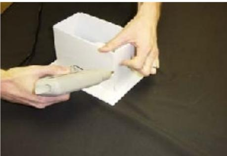
Here you can see we are using hot melt adhesive to glue and seal the seam of our mold box. We will also use the hot melt to seal all the edges of box to the base just in case the silicone were to seep down between the box and the clay. This will prevent the silicone from leaking. You can also use super glue, caulk, epoxy, clay, tape, or any other material to seal your mold box shut. Just make sure it is sealed tightly.
