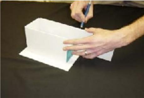
Here you can see how we are sizing the mold box right around the base of the clay. We simply score through one side of the corrugated plastic and bend it around the base. We then seal the inside of the mold box by smearing the clay tightly against the box. This ensures us the mold box will not leak. It is a good practice to double check this before pouring your rubber. An extra minute double checking the mold before pouring could save a costly mistake and a real mess.
