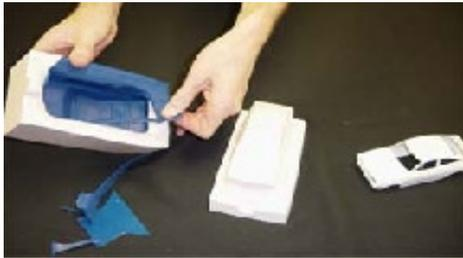
Next simply remove the flash from the car. The flash is the thin film of resin that was stuck and cured between the two halves of the mold.
