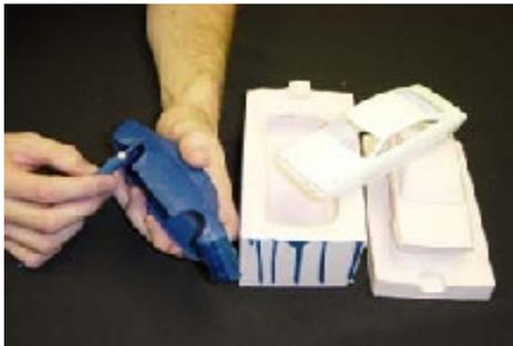
It is much easier to trim the excess flash away when the material is still setting up (within 5 minutes of demolding). If you can trim the car with a sharp Excel or Exacto knife while it is still semi flexible, it will make it much easier. If you wait 15 minutes or more before trying to clean up the casting, the material gets very hard and does not trim as easily.
