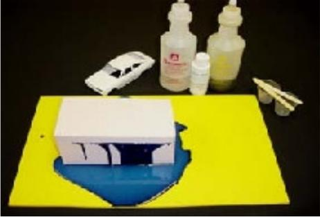
The Alumilite Regular has 90 second work time and a 3-7 minute demold time. With a thin walled car you will want to wait closer to the 7 minutes before demolding. You can wait longer if you wish. The longer you wait, the harder the casting will be. The Alumilite Regular features a color change to at the 90 second point to notify you when the work time has ended. You can see the color difference in the blue as it begins to harden.
