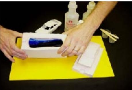
Once you've poured all of the resin into the mold, simply rotate the mold to allow the resin to coat every side of the mold. Important Note: Make sure to work over a piece of scrap plastic or wood. Or make sure to mold release a table or work area so the resin will not adhere to it. Do not spill or squish the resin over any type of carpet, fabric, or clothes. The resin will stain and once hardened will not come out.
