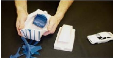
Then flex the bottom half, the female side, of the mold and remove your perfectly cast replica of your original. You can see how flexible the High Strength 2 silicone rubber is and how far you are able to stretch it without harming the mold. The tear strength is very high and you would not be able to tear this mold without cutting it with a sharp knife.
