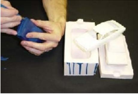
Once cured the Alumilite Regular can be painted, machined, sanded, polished, electro plated, and even heated back up to be reshaped (works best in thin sections). Take your time finishing up the trim work on your cast replica. The better job you did claying up the original, really saves you the time in these finishing steps as you will notice a significantly cleaner and smaller seam line.
