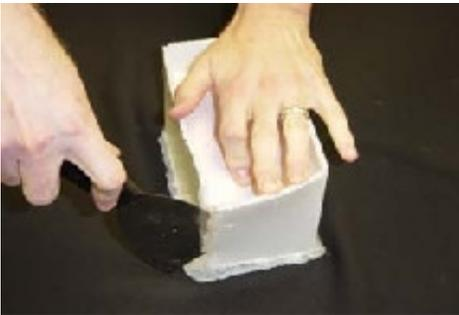
Let the silicone set up overnight. Using a dull or putty knife, break away the mold box from your two halves of your mold.
