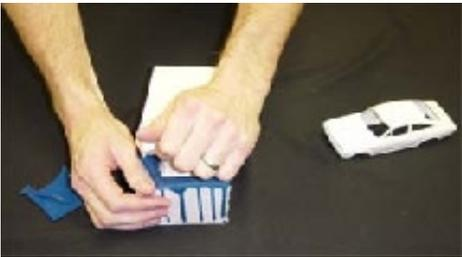
You are now ready to demold your cast piece. Simply start from one end and flex the male or top portion of the mold until you can remove it. You may have to simultaneously flex the lower half depending on the depth of undercut you have on your piece.
