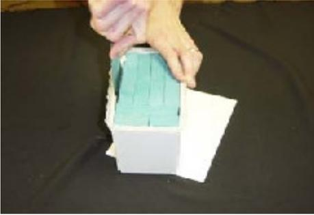
Start removing the clay from the mold box and your original using a dull knife or putty knife. It is very important not to move or break the seal of the part nestled into the first half of your silicone mold.
