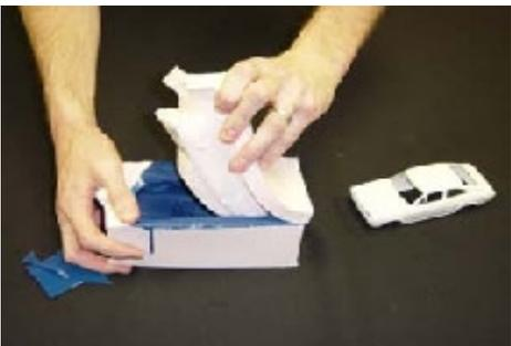
Here you can see the male portion of the mold being removed from the cast piece and the female half of the mold.
