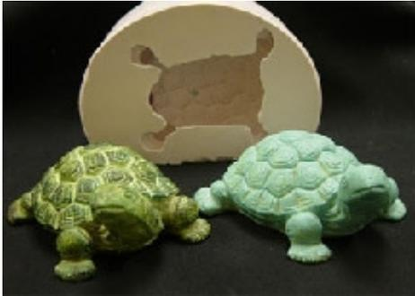
Here you can see the original turtle along side of our slush casting that was backed with the 610 Foam. The original turtle on the left used approximately 40 ounces of resin, whereas the slush cast turtle on the right used 4 ounces Alumilite resin and 3 ounces of the 610 Foam. Therefore we cut the amount of resin used from approximately 40 ounces to 7 ounces.
