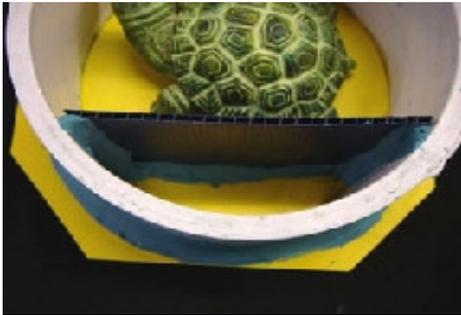
As you can see we fastened the turtle in the mold box off center to reduce the amount of wasted space. To eliminate the wasted space we cut a piece of Aluilite Corrugated Plastic and sealed it with Aluilite Synthetic Clay. We also sealed the PVC pipe to the base using the synthetic modeling clay.
