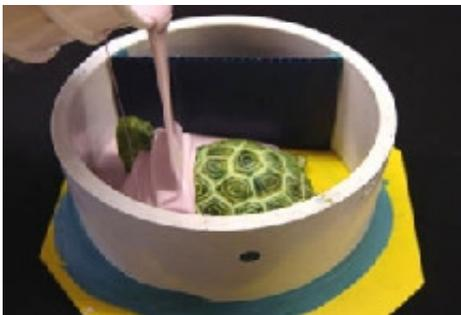
Once the mold box has been sealed, mix and pour the silicone rubber. We have chosen to use the Aluilite High Strength 3 silicone rubber because of its low durometer and high tear strength which will aid in demolding the piece.
