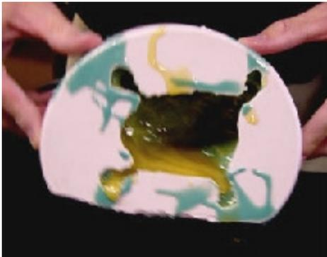
Once we've mixed equal amounts of the 610 Foam, we poured it into our mold. Because of the fine detail and multiple layers of the the turtle's head, neck, body, and feet we slushed cast the foam a couple of times to make sure we had all of the surfaces in the mold covered.
