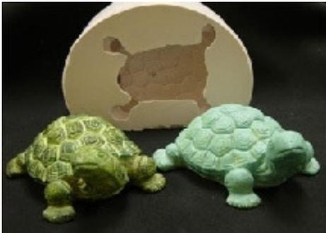
To slush cast is to pour a fraction of the amount of resin into your mold (typically of a bigger piece that has a lot of volume) and coat the sides with it by rotating the mold while the resin cures. Once the sides are coated, you can back fill the piece or leave it to be hollow.
