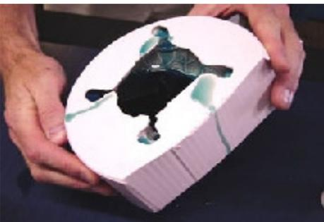
This is where the slush cast term comes from. The amount of mixed resin is a fraction of the amount required to fill the mold. Next, we pick up the mold and continually tilt it, forcing the resin to coat all of the sides in the mold. We continue to slowly slush the resin around in the mold until the resin sets up (approximately 2 minutes with Alumilite Regular).
