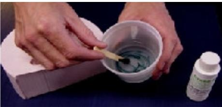
We recommend warming your mold prior to casting to ensure the thin section of the slush cast cures properly. Here we are adding a touch of green dye to the A side of Alumilite Resin to give us a light green finished color. Once we've mixed the green dye in thoroughly, we add the B side to the green A side.
