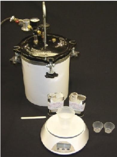
These are the items we used to mix and pressure the Clear: Pressure Pot, shop air, Alumilite Clear, Alumilite's Gram Scale, a 6 oz mixing cup, two 1 oz cups, and a stir stick.
