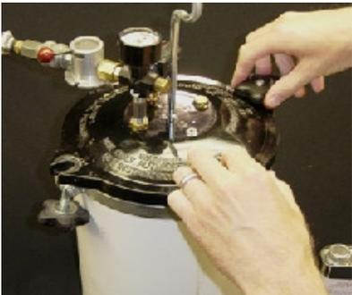
It is very important to fasten all of the knobs down tightly to the lid. The red handle on our tank is a ball valve, which allows us to hold the pressure within the tank while disconnecting the air source after it has reached the proper air pressure in the tank. In addition, the ball valve allows you to slowly add pressure to the tank without splattering the resin out of the cup/mold. We recommend installing a ball valve if your Pressure Pot does not have one.
