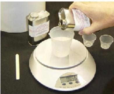
Measure Alumilite Clear using a mix ratio of 1:1 by weight. It will not cure properly if you mix it by volume.
