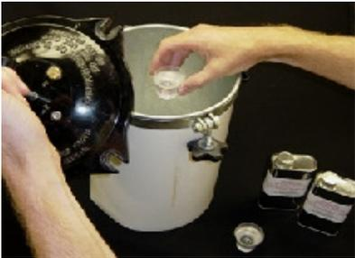
Here we are placing one of the cups in the Pressure Pot to be pressure cast.
