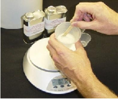
Once measured properly, mix thoroughly. The open time is approximately 6-7 minutes. Be sure to scrape the sides and the bottom of the container. It is very important to make sure you get the mixed resin into the pressure pot and to apply the air pressure prior to the resin starting to gel.
