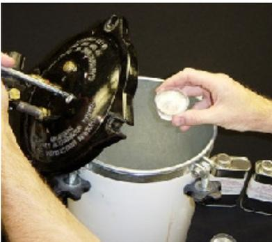
We remove our Alumilite Clear cup from the Pressure Pot and see no air bubbles in the poured cup at all.
