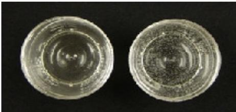
Here you can see the difference between the castings on the left that has been pressure cast compared to the cup that was just mixed and poured without the use of pressure. The cup that was pressure cast does not have any air bubbles. The cup that was not pressure cast has hundreds of small champagne sized bubbles throughout the entire casting.
