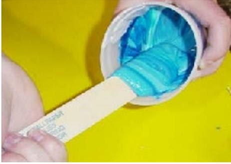
You are now ready to mix and pour the first half of your silicone mold. We used Alumilite's Plat 55 silicone mold making rubber because we wanted a more firm mold where the two halves of the align well. It also enables us to clamp or hold the mold together without distorting it. QuickSet mold rubber is another good choice as well as High Strength 2 if there is a little more undercut to your original. Plat 55 is thicker than QuickSet but has a much higher tear strength.
