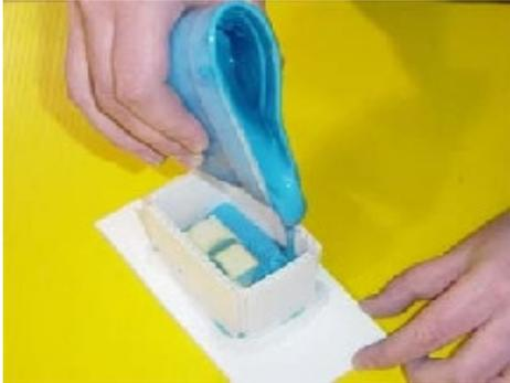
Once the silicone is mixed completely, pour it slowly into the mold box from one corner. Let the silicone flow around the master naturally. Avoid pouring the silicone directly over the master to reduce the chance of trapping air pockets against your original.
