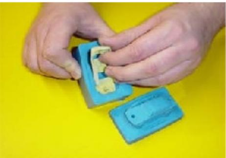
Allow the second batch of mold rubber to set up overnight. Remove the mold box and separate the two halves of the mold. Then simply remove your original and you are ready to start pouring slot car bodies.
