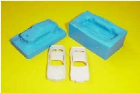
This How To process will walk you through step by step the procedure for making a two piece squish mold and casting a slot car.
