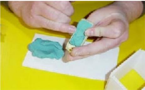
Using Alumilite's Synthetic Modeling Clay we filled in the car body with clay to act as one half of the mold. This prevents the mold making silicone from flowing inside the car and removes any undercuts. We will use the bottom edge of the car as the parting line.
