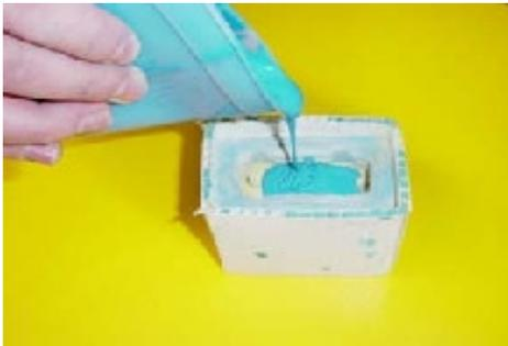
Demold the first half (completely remove all the clay), apply Alumilite's Rubber to Rubber Mold Release, Alumilite's UMR or a thin layer of Vaseline to ensure the two halves of silicone do not bond to each other. Then mix the second batch of silicone and pour the second half of the mold.
