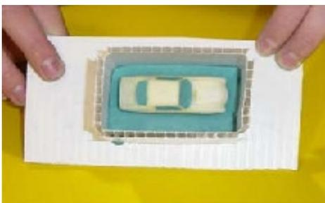
Once the car has been completely clayed up, assemble and seal the mold box using the same modeling clay, hot melt glue, super glue, or any other sealing material.
