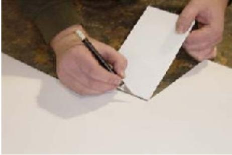
Once you have the original perfect, decide what material you are going to use for your mold box. You can use styrene, corrugated plastic, wood, metal, foamcore, posterboard (shiny side), or any other non-porous material. Here we chose to use styrene for the base and corrugated plastic for the side walls of the mold box.
